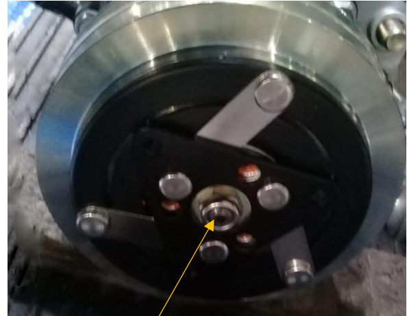
Turn the compressor clockwise using the wrench with a socket 13 or 14 (depending on the compressor installed).
