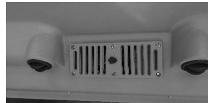
Air recirculation blinds
